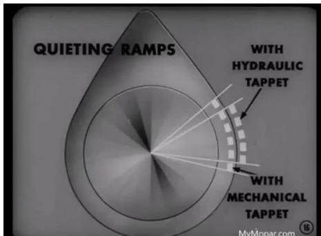
Pro of having More preload/tighter lash: gives an engine more bottom end or torque.
