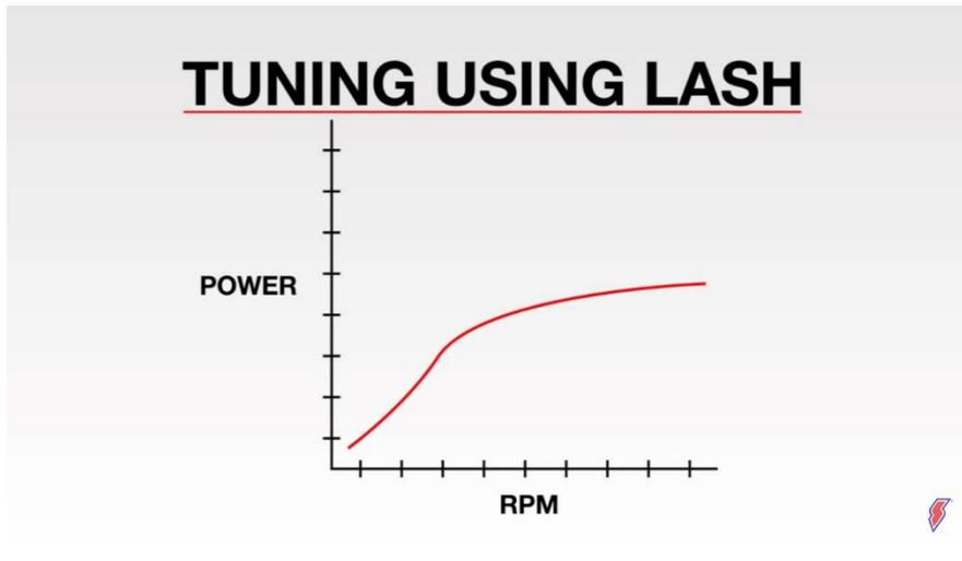
Con of having more preload/tighter lash: too much can hang open valve and smack piston. Loss of horsepower on top end.
