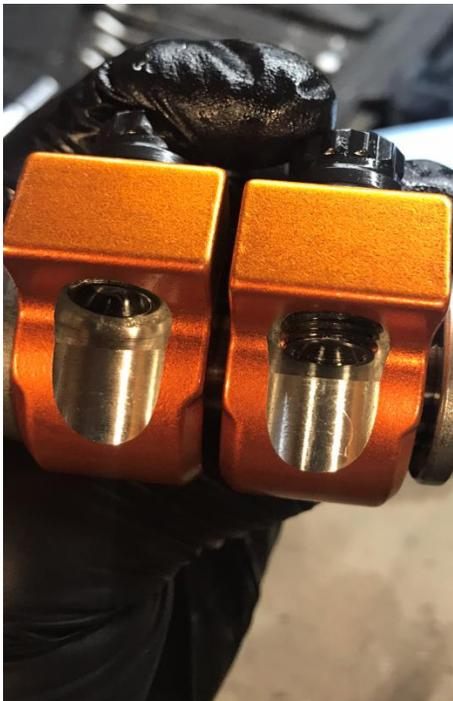
Same as above, If you put the correct amount of preload on the lifter, but you aren't achieving the correct thread level on the bottom of rocker, then your pushrod is too long or short. Harland Sharp rockers must have 2min-3max threads showing at the bottom for proper oil passages.
