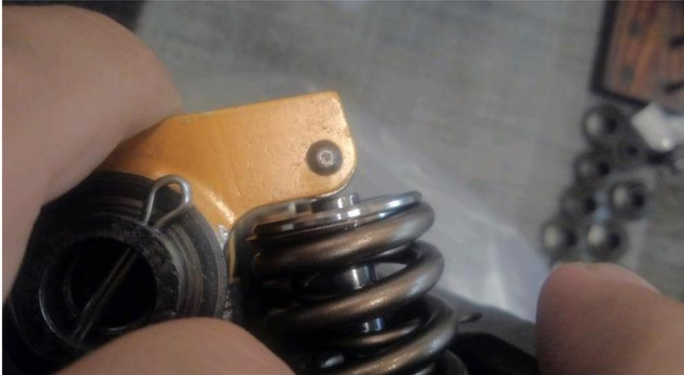
If you put the correct amount of preload on the lifter, but the rocker isn't centered, then your pushrod is too long or short. This goes for any style rocker.
