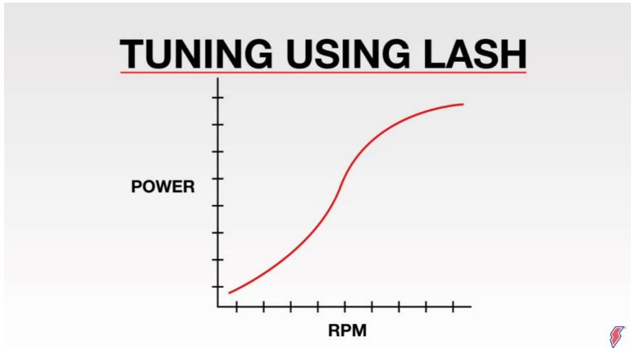
Con of having less preload/greater lash: decreases duration of cam, and in essences makes the cam smaller. Also, can cause engine to be noisy and loose control of valve train. Overall, it's harder on the engine.
