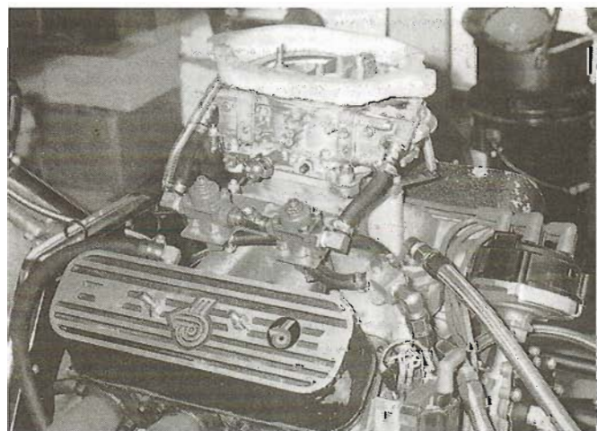
The Stage II manifold (25500029) in action on a development dyno. This piece has an aluminum 4-barrel design with a square-bore carburetor mounting flange and no heat crossover passage. Note the use of a pressure regulator for each of the float bowls. Foam at the top of the carburetor seals it to a plenum.
